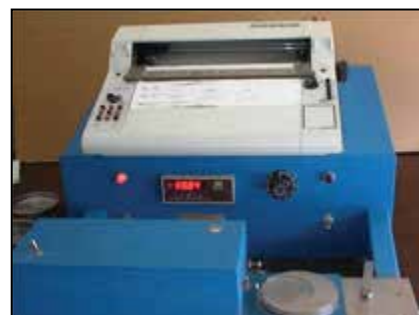
FIGURE 2. The Jenike Shear Test Method, for determining a solid's flow properties, is used in an ASTM standard
