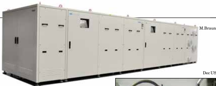
FIGURE 4. The MBRAUN 3000-IGMS is said to be the world's largest and most powerful inert-gas purifier
