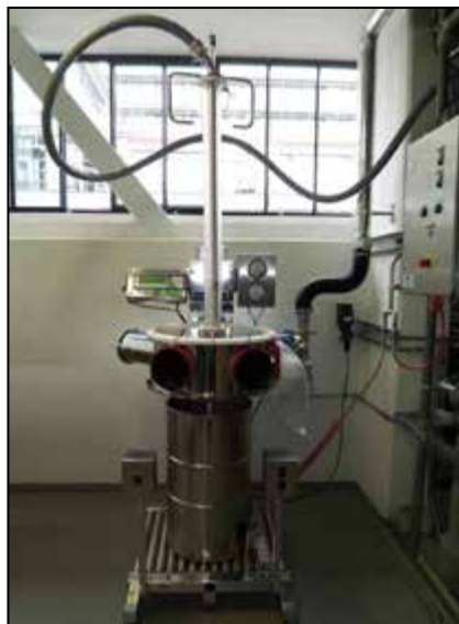
FIGURE 5. The DCS is a stainless-steel cylindrical glovebox with glass cover and two glove ports
