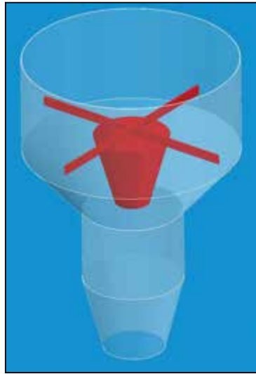
FIGURE 12. Cone-in-cone devices are designed to convert funnel-flow patterns to mass-flow solids flow
