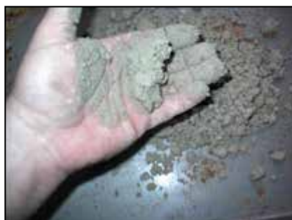
FIGURE 1. Many solids exhibit caking or packing properties when under pressure, such as that seen in a bin or silo
