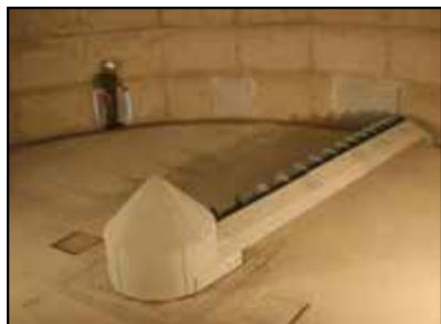
FIGURE 7. Traveling-auger unloaders work well with woodchips, biomass and granular or flaky materials
