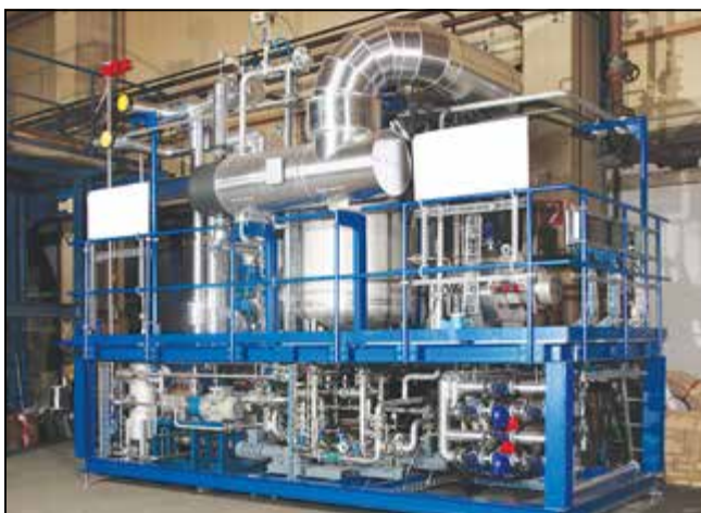
Thin-film dryer unit from GIG Karasek
